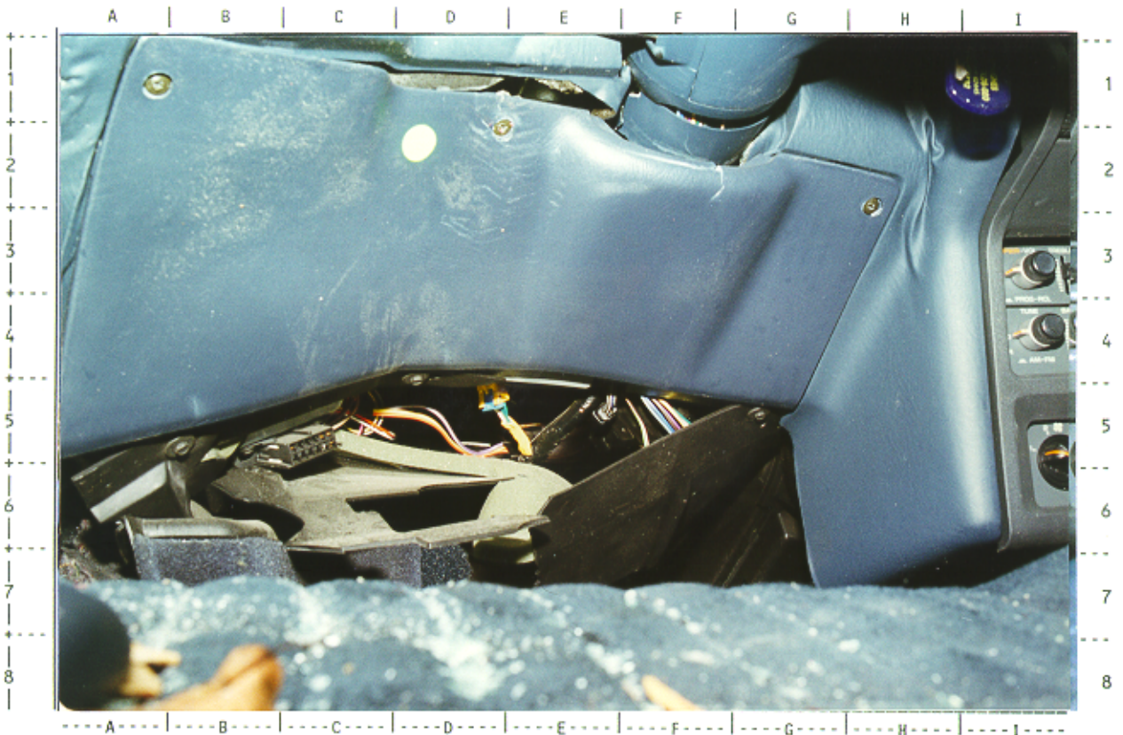
# 56 -- Interior of 1991 Chevrolet Corsica's lower left dash area viewed from left showing driver's left knee contact with knee bolster
